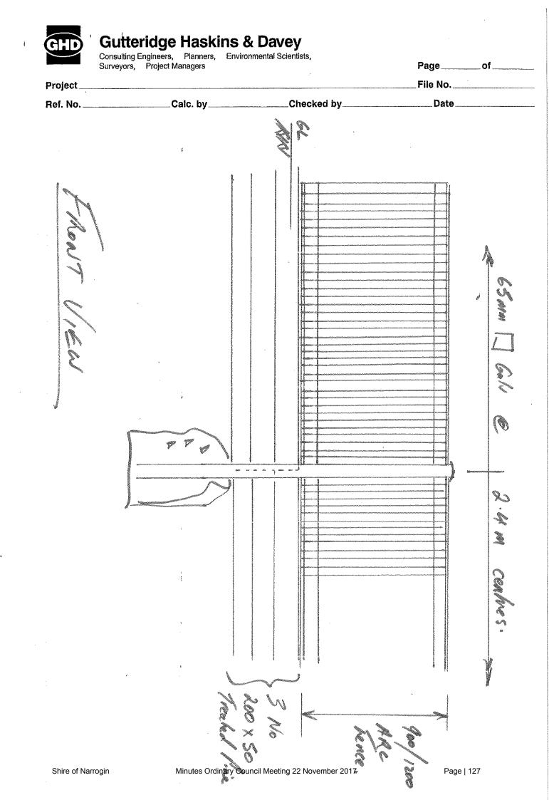
**Gutteridge Haskins & Davey** Consulting Engineers, Planners, Environmental Scientists, Surveyors, Project Managers Page\_\_\_\_of\_\_ Project. File No. Ref. No. Calc. by\_ Checked by..... Date SIDE VIEW 900/1200 AAC FEACE. 3 No 200 × 50 Slagers 65 mm D Gal Post TON GREEN -/co Ma 50 Varies Hoo - SSom Lower GREEN KKVI 5.2 Nomina 1 600m Depth footing Minutes Ordinary Council Meeting 22 November 2017 Page | 128 Shire of Narrogin Gutteridoe Haskins & Davev Ptv I td
