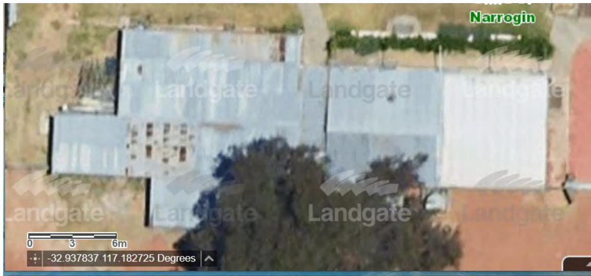
FIGURE 4; AERIAL PHOTO OF SHED. NOTE THE TWO AREAS OF RUSTING ROOF.
