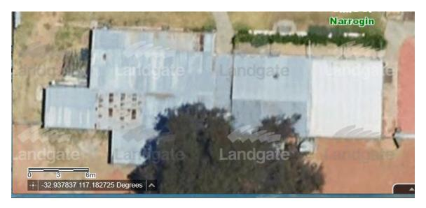
Figure 4; Aerial Photo of Shed. Note the two areas of rusting roof.
